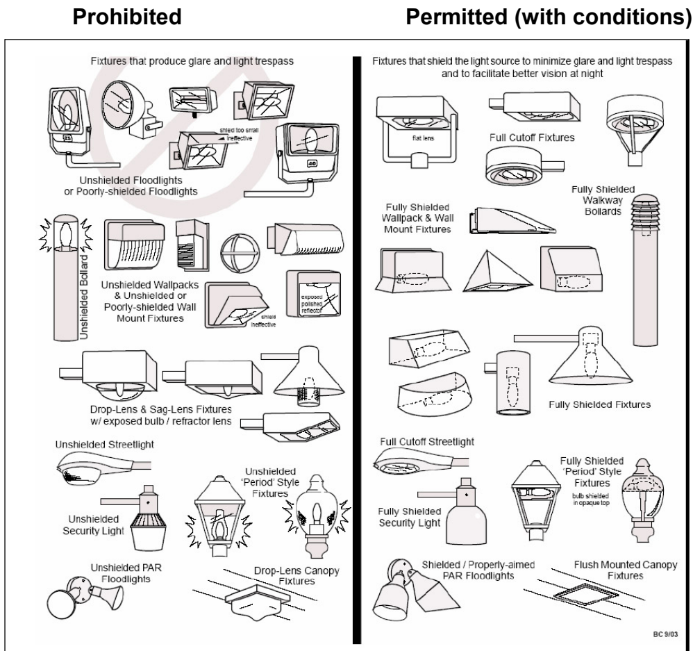
Figure C (Examples of Prohibited and Permitted Outdoor Lighting)
